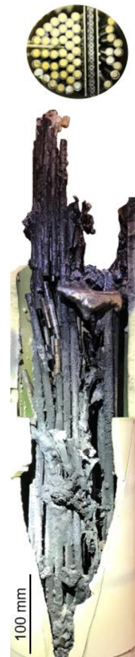
Fig.1 Post-test appearance of the CMMR-4
