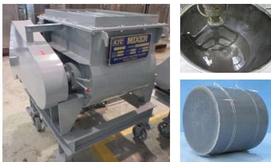
Figure 2 Experimental equipment and solidified geopolymer
