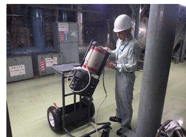
Fig.3. ISOCS measurement for Reactor building wall and floor.
