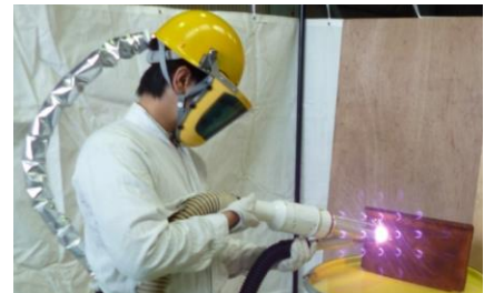
Fig. 1 Portable laser paint removal device
