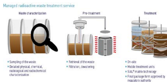
Figure 1 SIAL ® solidification treatment process
