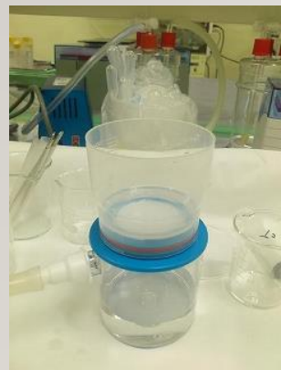
Filtration to separate particles from liquid
