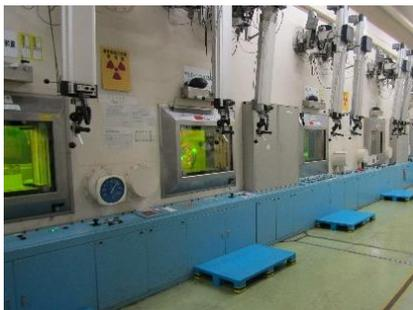
Hot cells (Concrete cells)
