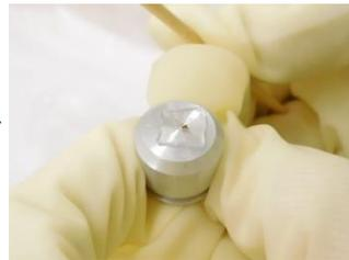
Sample preparation for SEM (Scanning electron microscope)
