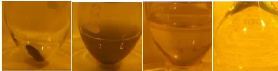
Before dissolution    Addition of nitric acid    After dissolution    After solid-liquid separation
