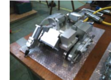
Inspection Robot for Lower part of S/C
