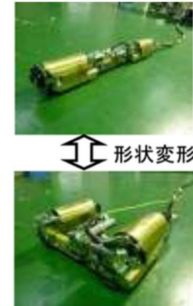
PCV Inspection Robot PMORPH
