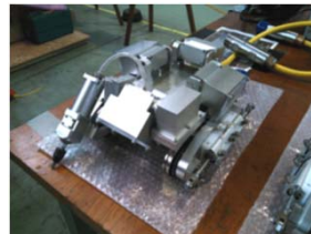
Inspection Robot for Lower part of S/C
