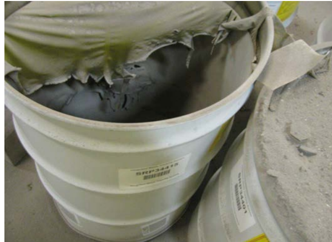
Ruptured drum at INL
