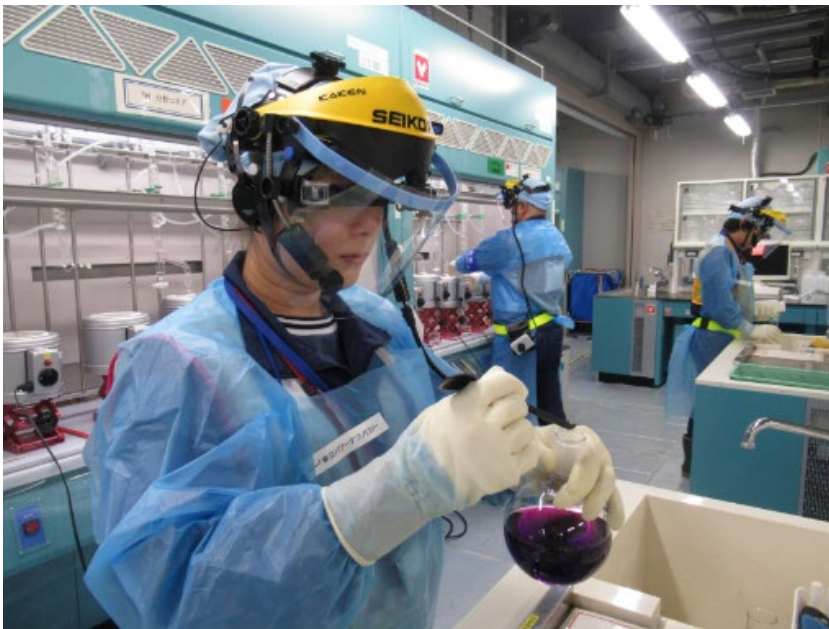
Chemical manipulation prior to tritium analysis(chemical analysis building)
